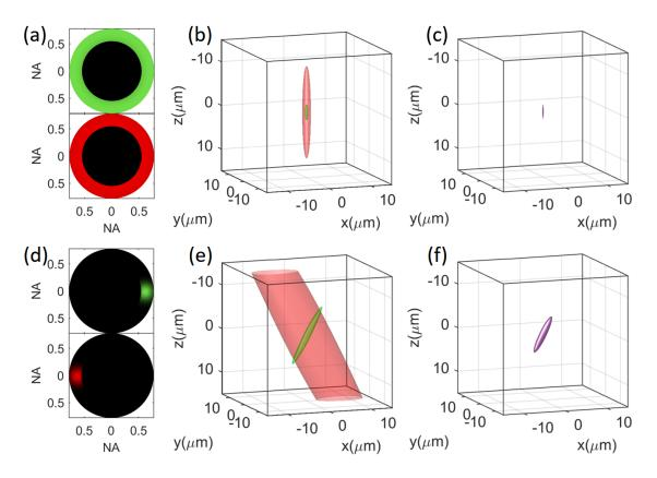
**Figure S1. The numerical simulation of the foci and the chiral SFG point spread function.** First row depicts collinear modality: (a) laser intensity at the objective lens pupil; (b) foci; (c) chiral SFG PSF. Second row depicts noncollinear modality: (d) laser intensity at the objective lens pupil; (e) foci; (f) chiral SFG PSF. The colors green, red, and purple are used to represent wavelengths of 520 nm, 3274 nm, and 448.7 nm, respectively.
